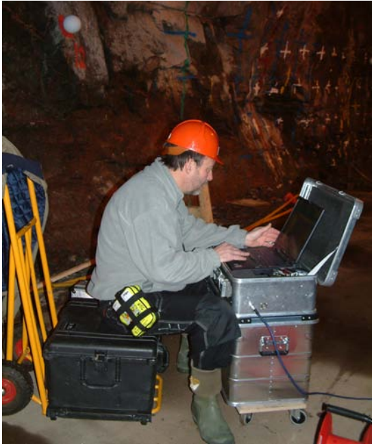
TASQ-tunnel, the computer work by ATS to collect laser scanning data
