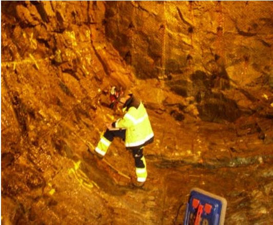
Mapping of the tunnel floor of the TASQ-tunnel
