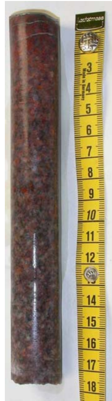
Drilling of sample cores from matrix rock surrounding the test section in the small diameter extension borehole (left) and sample core A6, about 18 cm long, drilled from the fracture surface on the core stub (right).
