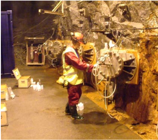
Operation of the five miniature canisters
