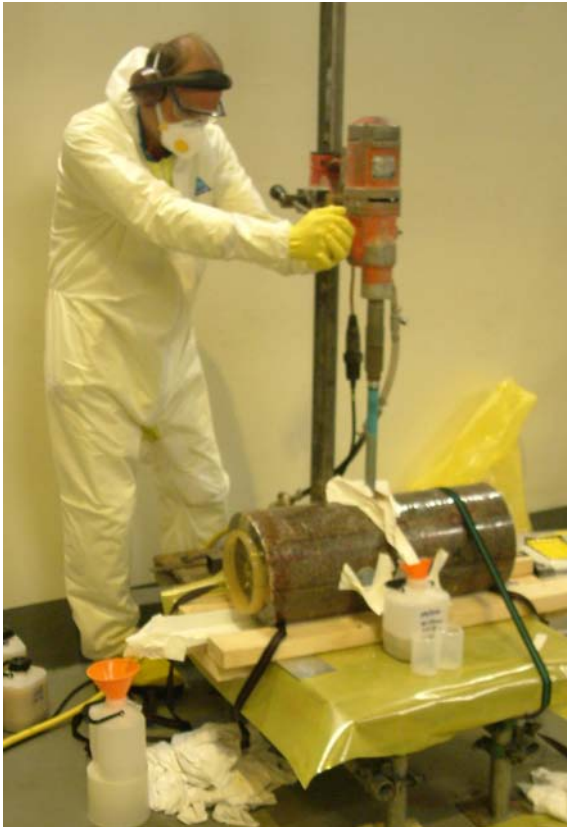
Drilling of sample cores from matrix rock surrounding the test section in the small diameter extension borehole (left) and sample core A6, about 18 cm long, drilled from the fracture surface on the core stub (right).
